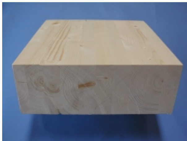
Figure 3: Melamine-Urea-Formaldehyde (MUF) glued specimen.
