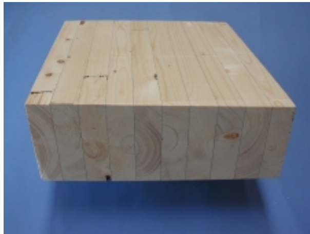
Figure 2: Phenol-Resorcinol-Formaldehyde (PRF) glued specimen.
