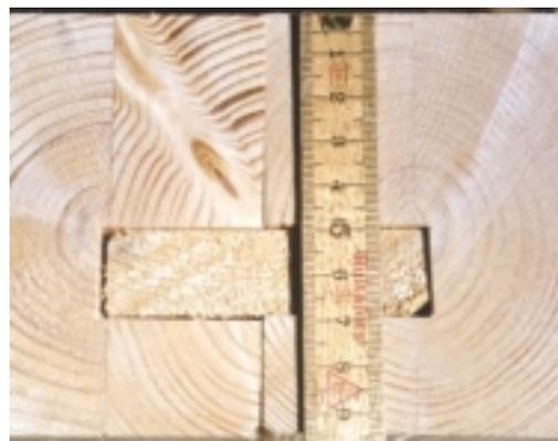
Figure 4: Cross-sectional view of glued solid wood elements with the used tongue groove connection.
